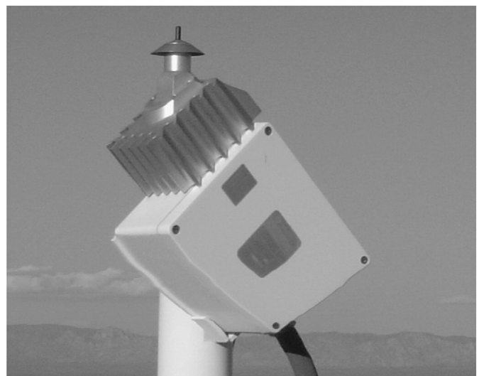
Fig. 13. Probe-style ice detector for measuring freezing rain and freezing drizzle (courtesy author).
