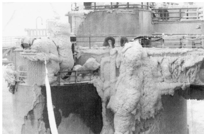
Fig. 2. Superstructure icing on the semisubmersible Ocean Bounty in Alaska (Courtesy U.S. Minerals Management Service).
