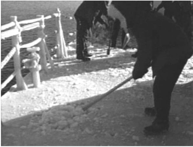
Fig. 11. Manual deicing of superstructure ice with wooden baseball bat on forecastle deck of U.S. Coast Guard Cutter Midgett (from video courtesy author).
