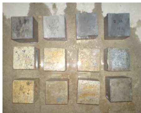
Figure 10. Specimens in lime saturated water, 5% Na 2 SO 4 and 5% MgSO 4 .
