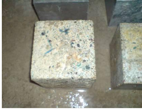
Figure 11. Deterioration on cubic control specimen after 3 months exposure to 5% MgSO 4 .
